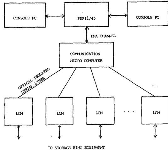
FIG. 4 BLOCK DIAGRAM OF HESYRL RING CONTROL SYSTEM
