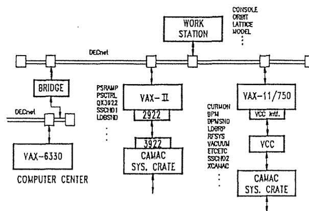
Figure 2 The upgrade of BEPC control system
